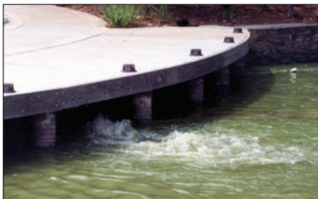
Minimum operating depth for Tritons is 3ft or 92cm, while Sub-Tritons require 2.5ft or 76cm of water depth.
